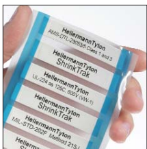
Step 1 Print with thermal transfer printer
